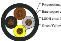
Polyurethane/PUR outer jacket Bare copper conductor LSOH cross-link polyolefin insulation Green/Yellow wire
